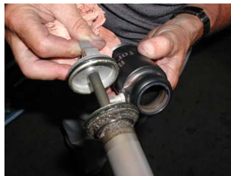
Very extreme example of removal of dirt inside (mud)
